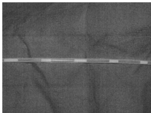
Figure 5. Miniemulsion using metered nitrogen to induce isolated plug flow.
